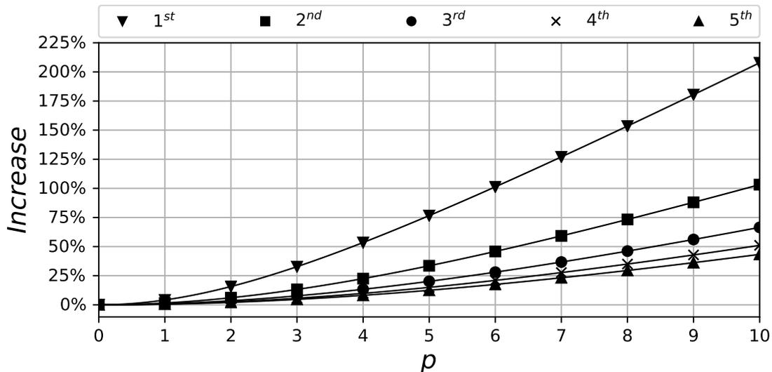
Figure 5: Increase in the natural frequencies of a beam on Pasternak ( $e = 5$ ) foundation considering the parameter  $p$  (FEM - 70e).
