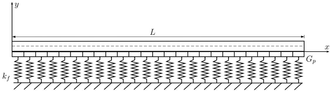
Figure 1: A beam on a Pasternak foundation.
